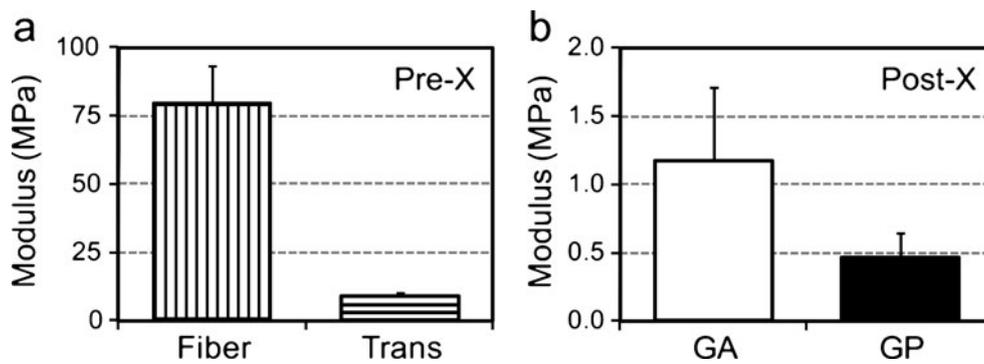
**Fig. 3** Mechanics of type I collagen nanofibrous scaffolds before and after crosslinking. **a** Tensile modulus of dry pre-crosslinked (*pre-X*) collagen scaffolds in the fiber and transverse to the fiber directions. **b**
